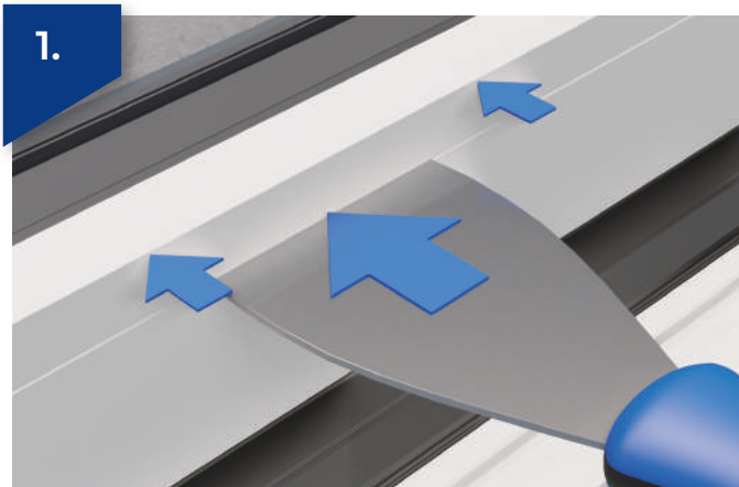
1. Push on upper edge of bead to tilt it backwards to allow you to slide a tool between the bead and sash profile.
