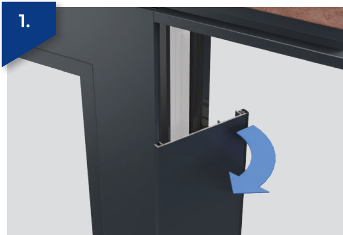
Remove interlock on fixed sash.
