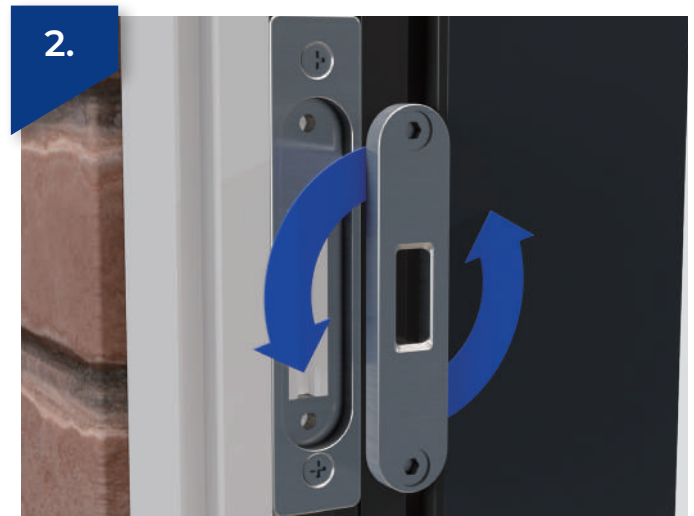
3mm adjustment is available by turning faceplate through 180°.
