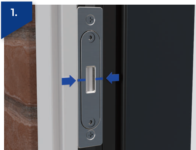
Should be set at nominal with the two lines matching. Adjustment can also be made using a T25 driver.
