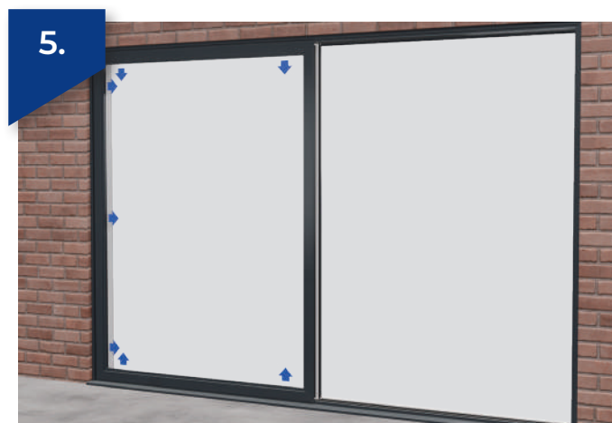
Remove fixed sash screws in glazing area.
