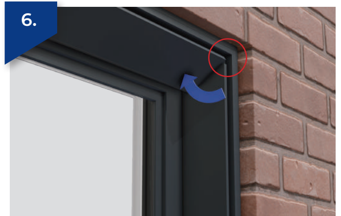
Fit jamb trim to head. Do not forget to fit the jamb trim corner shrouds top & bottom, handle side only (indicated above in red).
