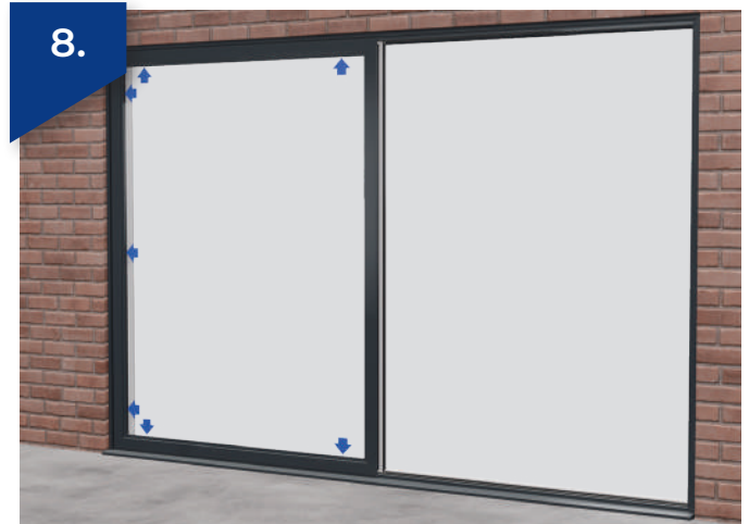
8. Fix 100mm from corners at no greater than 1000mm centres using 4.8 x 65mm long screws.
