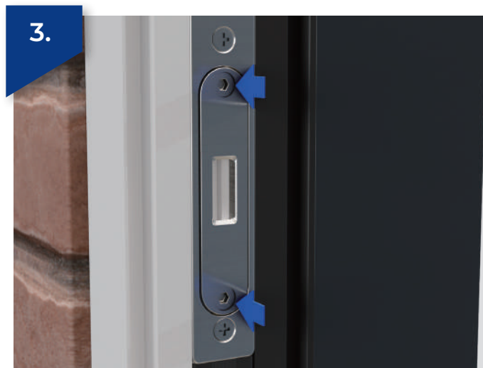
The keep is also adjustable in and out. Use a T25 driver to adjust +/- 2.5mm
