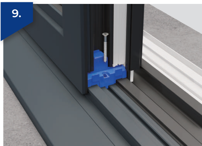
9. Fix the fixed sash corner dams (silicone behind before fitting) using a 3.9 x 35mm screw. Repeat top & bottom.
